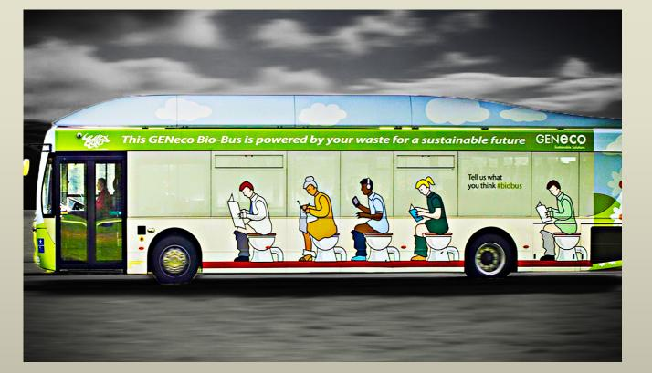
UK's BioBus, a 40-seat bus that runs on biogas generated from the treatment of sewage sludge and foodwaste.
