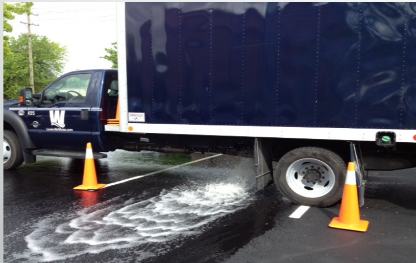
Meter testing via truck mounted apparatus (Courtesy of Louisville Water Company)
