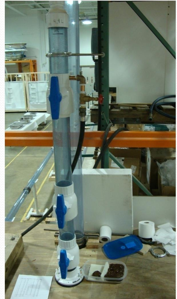
Photo: Surge Injector installed on apparatus flush stand
