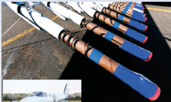
Burn-in-place flares are mounted on the aircraft wing to disperse silver iodide in a cloud.
