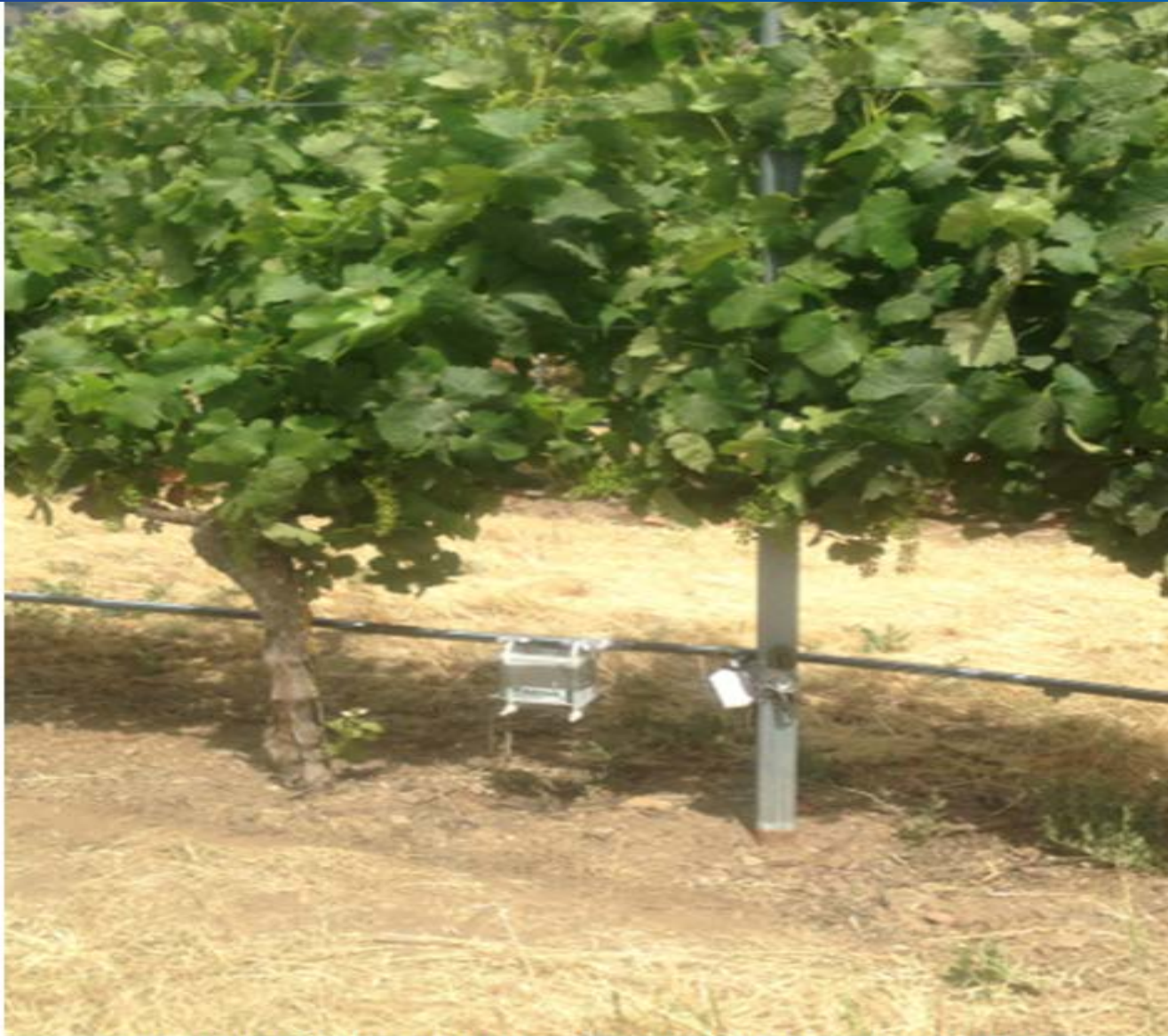
Figure 9: irrigation gauges installed under the water emitter
