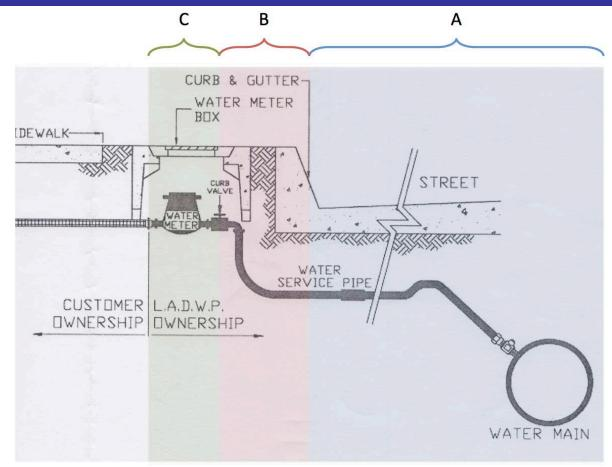
A - Main Breaks and Service Leaks between the Curb and the Main Source: GIS and Trouble Board
