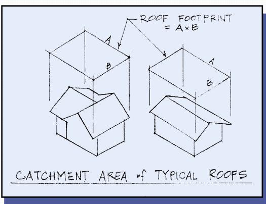
Regardless of the pitch, the shape, or the complexity of the roof surface, the overall footprint of the building determines the collection area.
