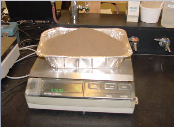
Fig1: Oven Dried soils being weighed.
