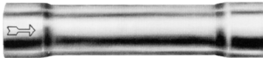
Dole Automatic Flow Regulator (actual size) 4 \frac{1}{2} " long with \frac{3}{4} " sweat connection
