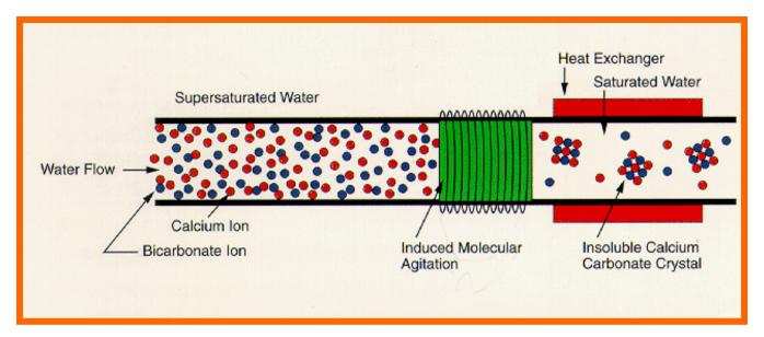
Pulsed low (60 Hz) & high (10-100 kHz) frequency EM fields
