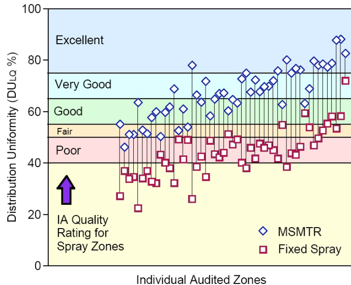
Figure 4. On average, DU improved by 23 points after conversion to MSMTTR sprinklers.
