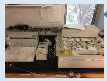
Nitrate and ammonium is extracted from samples using 1M KCl and then run on a Lachat Quikchem 8500 flow injection analyzer
