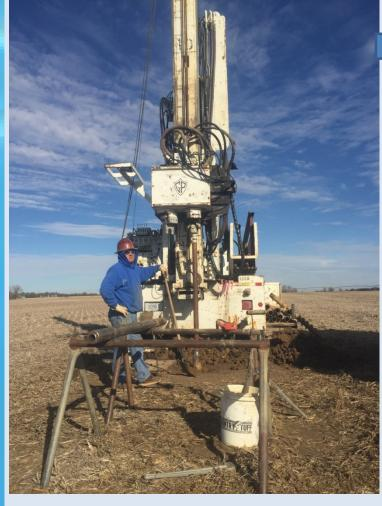
Continuous cores of the vadose zone are collected using a hollow stem auger drill rig. Samples are collected before planting and after harvest from farm land.
