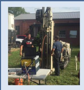
Recently, a hydraulic profiling tool (HPT) system was purchased for use with the school's Geoprobe. The HPT measures water injection pressure with depth and helps determine formation permeability. It can also measure saturated hydraulic conductivity below the water table.
