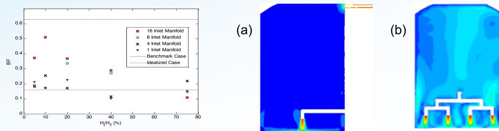
• Velocity contours show that a 16-manifold inlet (b) vs. a single elbow inlet facing downward (a) dramatically reduces the amount of dead space in a vertical cylinder tank.
