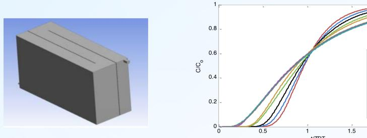
The ratio of baffle opening length ( $L_{bo}$ ) to tank length ( $L_T$ ) is important, as well as channel width ( $W_{ch}$ ) to  $L_{bo}$
