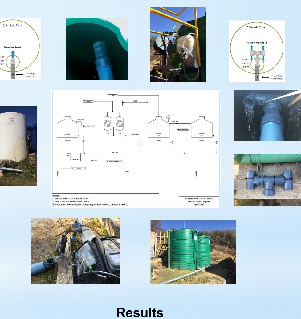
The baffling factor of the JoJo tank, 40-50% full, with a horizontal inlet with inline dosage was ~0.24. Once the modification was implemented the baffling factor increased to  $\sim 0.34$ , a 40% improvement.
