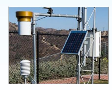
Advanced Weather Station Technology: IRWD uses the most advanced weather station technology, consisting of Campbell Scientific CR-10X Data Logger equipment, the same used by the California Department of Water Resources for the 100 California Irrigation Management Information System stations around the state.
