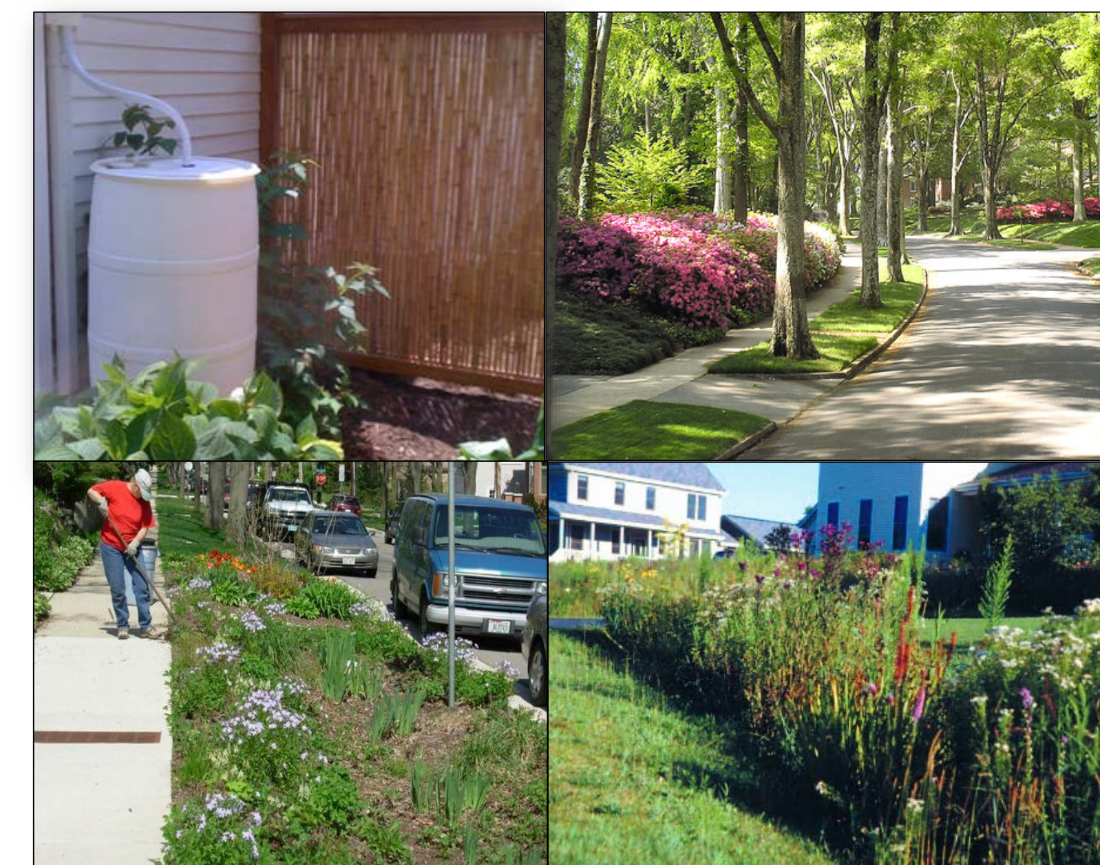
Fig. 4. Water management strategies implemented in Dane County and encouraged in the Dane County Natural Hazard Mitigation Plan. Clockwise from top-right: rain barrel, effective rain barrel, street terrace rain garden, development with bio-swale.
