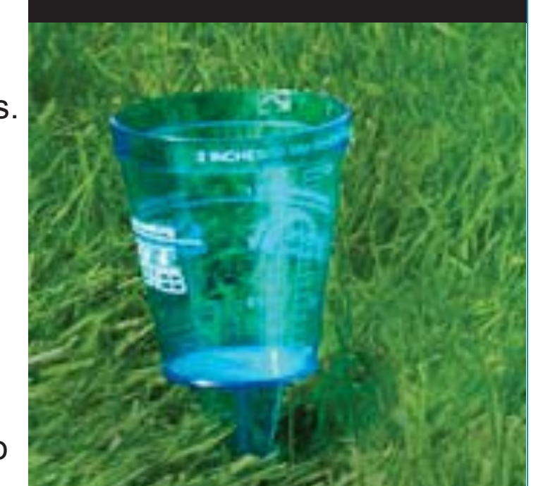
Picture 4—Green Grass Gauge—used to measure sprinkler output
