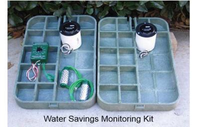
The purpose of the kit is to compare the total run time of irrigation valves that are controlled with either conventional or ET based controllers, to valves managed by plant demand. This is accomplished by selecting landscape properties
